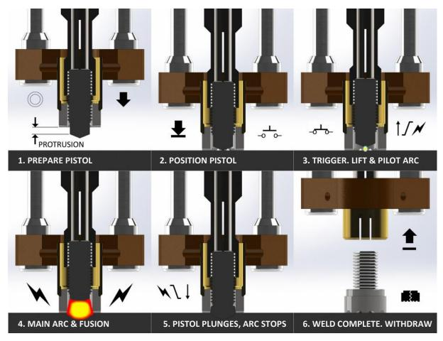
Having welded the stud, draw the pistol vertically off the stud. Failure to do this may cause the split tines of the chuck to splay out. This will result in the chuck and stud arcing together during subsequent welds.
