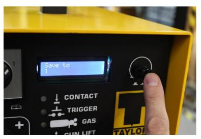
**NOTE!** It is not necessary to cycle through all 4 setting screens when making adjustments. If you wish to alter only one parameter. Cycle to the parameter screen you wish to adjust. Change it, then **PRESS & HOLD** the control knob to activate the "Save to" screen and follow the instruction above to save the settings to memory.
