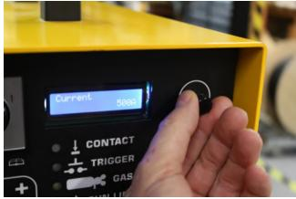
**TURN** the knob to set the required welding current. Once the desired number is reached. **PRESS & RELEASE** the knob to move on to the next parameter screen.
