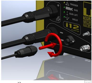
If optional shielding gas is to be used during welding. Attach the bottle supply to the controller via the front panel using a suitable self-sealing push-on socket.
