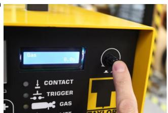
**TURN** the knob to set the required purging time. Once the desired number is reached. **PRESS & RELEASE** the knob to move on to the next parameter screen.
