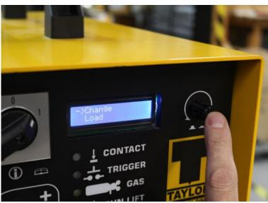
To adjust the welding parameters. PRESS & RELEASE the control knob and the display will change to show 2 options:
