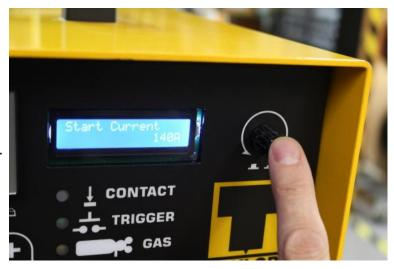
If you wish to go around the 4 parameter setting screens again **PRESS & RELEASE** the control knob to skip to the first screen (Current)
