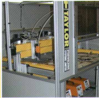
CNC system welding 2 components simultaneously
